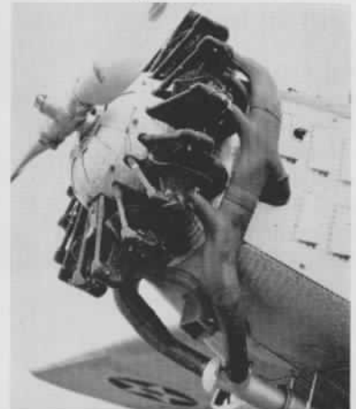
FIRST stainless manifolds went on a Chance-Vought O2U-4, left, and a Boeing F4B-1 in 1930, followed by stacks for a Ford tri-motor, center, and Loening amphibian, right.
