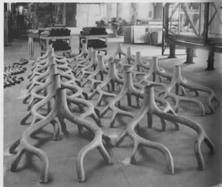
THE CONTRACT that saved a company. Part of Solar's first major order, $4000 of manifolds, stacks and heat exchangers for the Boeing 247, which literally rescued our payless, debt-saddled little plant in 1932, gave us a foothold.
