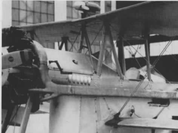
FIRST stainless manifolds went on a Chance-Vought O2U-4, left, and a Boeing F4B-1 in 1930, followed by stacks for a Ford tri-motor, center, and Loening amphibian, right.
