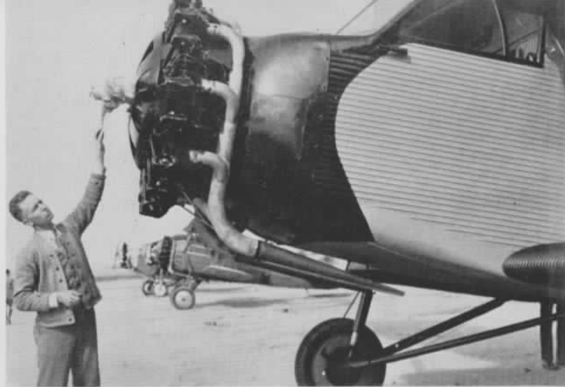
KEY TO THE FUTURE: Mechanic Red Perry took time off to pose with Solar's—and the industry's—first drophammer-formed manifold. Built of mild steel, it was mounted on the MS-1 after its first flight to replace original outside-purchased bent tubing ring.
