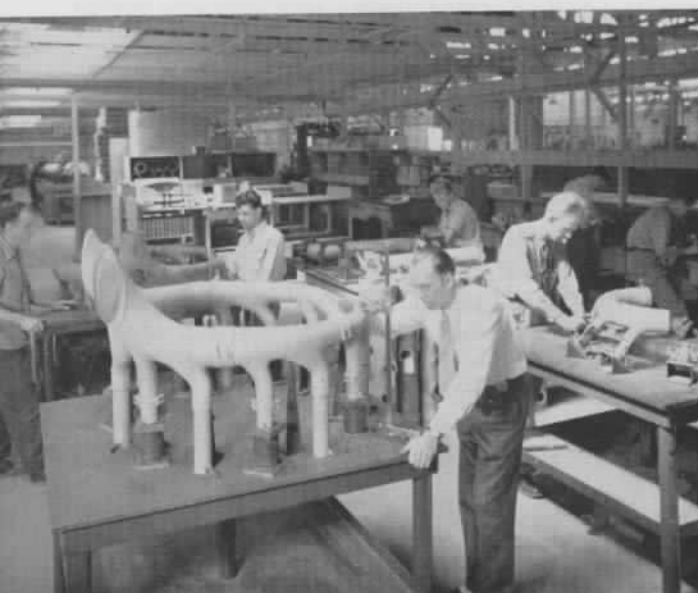
INSPECTION AND SHIPPING—1938: Closer tolerances were creeping into manifold production—.015 on most diameters, .005 on part flanges. Art Greer, right background, recalls that only two or three men knew how to read an NF-3 thread gage. Today's jet part tolerances average .003.
